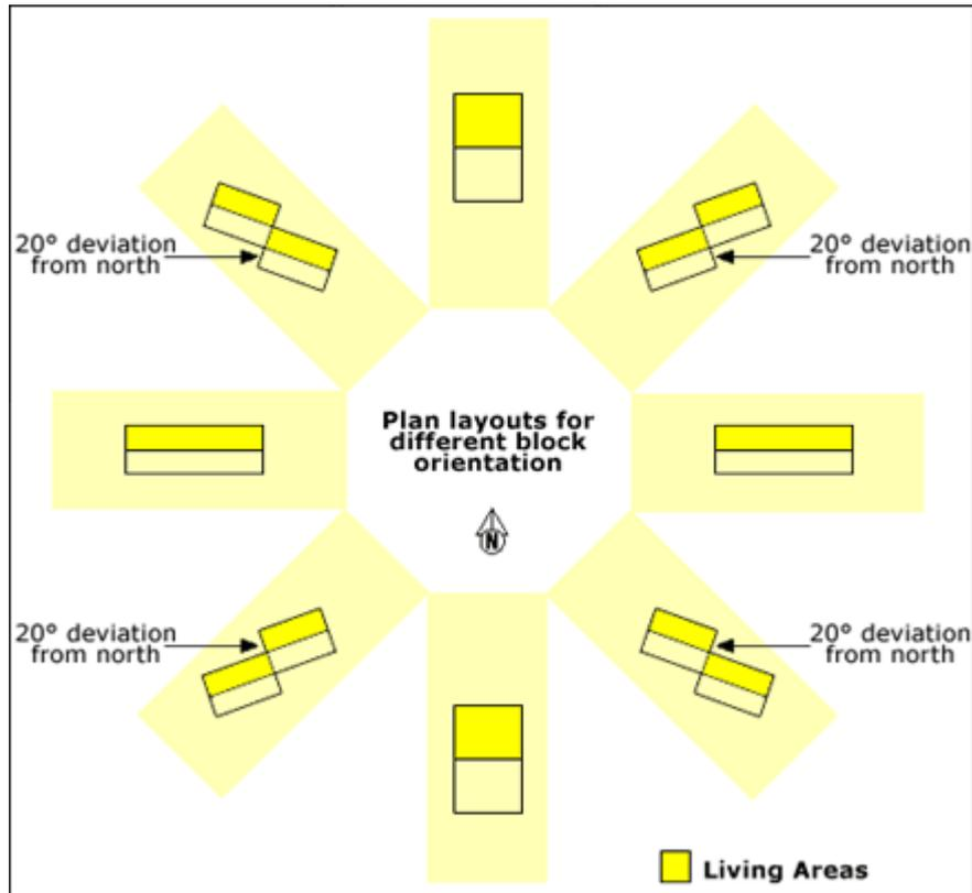
To achieve the design goal of optimal energy efficiency, an effective rule of thumb for a house in the southwest is to have north and south facing walls 1.5 to 2.0 times the length of east and west facing walls. This allows reasonable access to the winter sun from the north of the home, while reducing the exposure of walls and windows to early morning and late afternoon sun on the east and west sides of the home.
