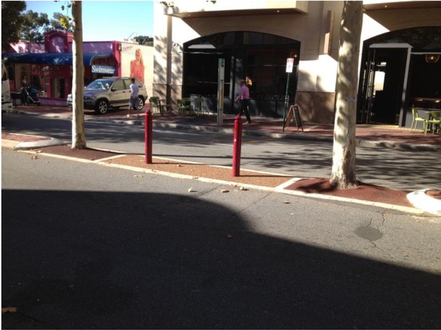
**Figure 11.** A combination of bollards (wood or steel) together with concrete kerbing generally provides sufficient protection for new trees in residential/ commercial streets with low traffic speeds i.e. <math>< 50\text{ km/h}</math>.
