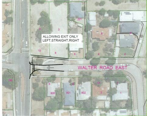
Existing Main Roads WA signalised intersection is proposed to be modified to permit traffic to exit from Walter Road East (east of the intersection) on their own phase
