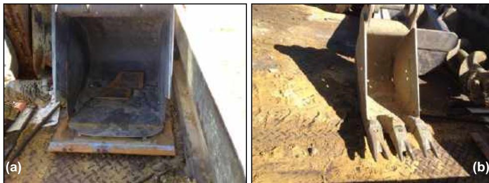
**Figure 5.** Where mechanical excavation is used outside the tree protection zone the selection of a toothless bucket (a) and use of a spotter can alleviate the extent of damage to the roots are they are revealed, compared with the toothed bucket (b) type which can significantly tear and damage roots.
