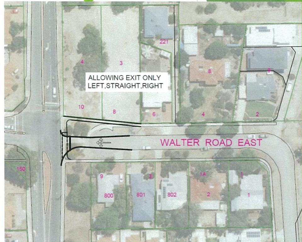
Existing Main Roads WA signalised intersection is proposed to be modified to permit traffic to exit from Walter Road East (east of the intersection) on their own phase
