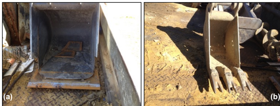
Figure 5. Where mechanical excavation is used outside the tree protection zone the selection of a toothless bucket (a) and use of a spotter can alleviate the extent of damage to the roots are they are revealed, compared with the toothed bucket (b) type which can significantly tear and damage roots.
