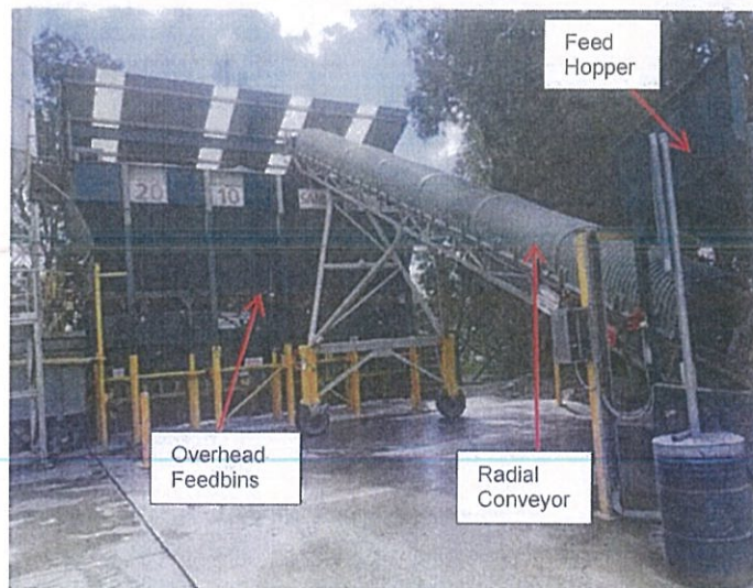
Figure 2: A typical radial stacker and conveyor delivering to overhead feed bins
