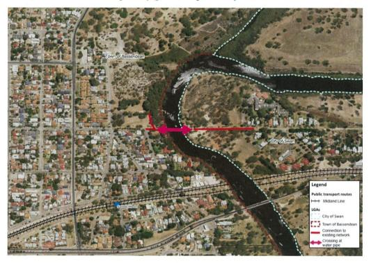
Figure 10 - Proposed water pipe pathway alignment
