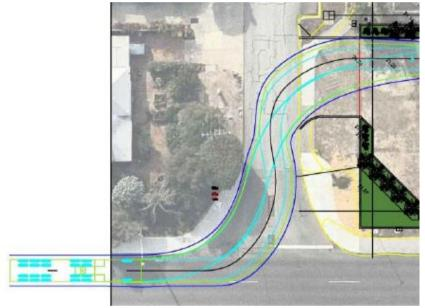
Figure 4: Fuel Tanker Turn Path Analysis (Page 8 of Transcore report)
