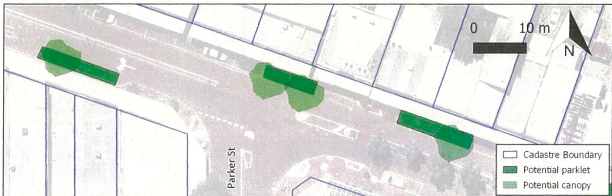
Figure 10: Example of the creation of parklets in reclaimed car parking bays. The shaded green polygons indicate the boundary of the potential parklet, and the semitransparent green polygons are potential canopy if broad crowned trees are planted within the parklet.
