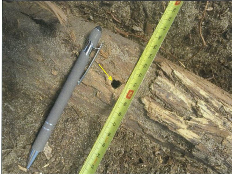
Figure 5. Closer inspection revealed an 8mm drill hole (see arrow) which is likely to be the probable entry point for the intentional application of herbicide.
