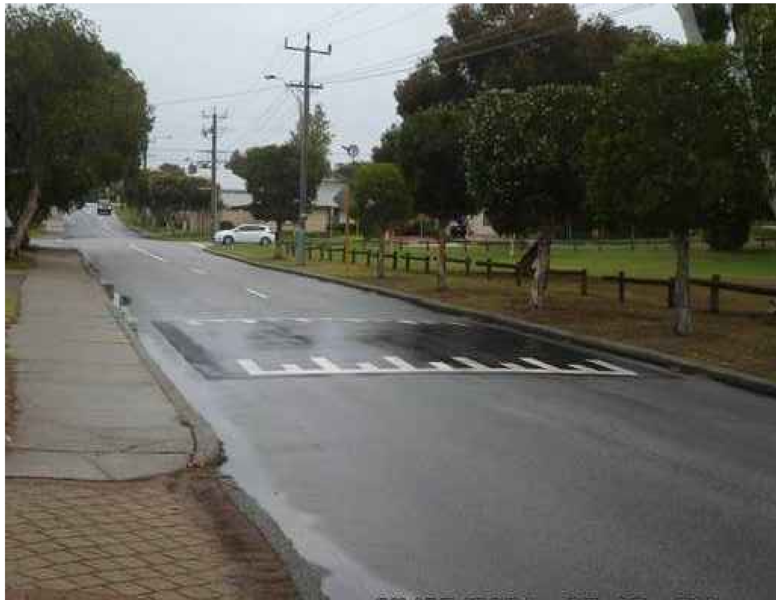
PHOTO EXAMPLE - ASPHALT SPEED PLATEAU
