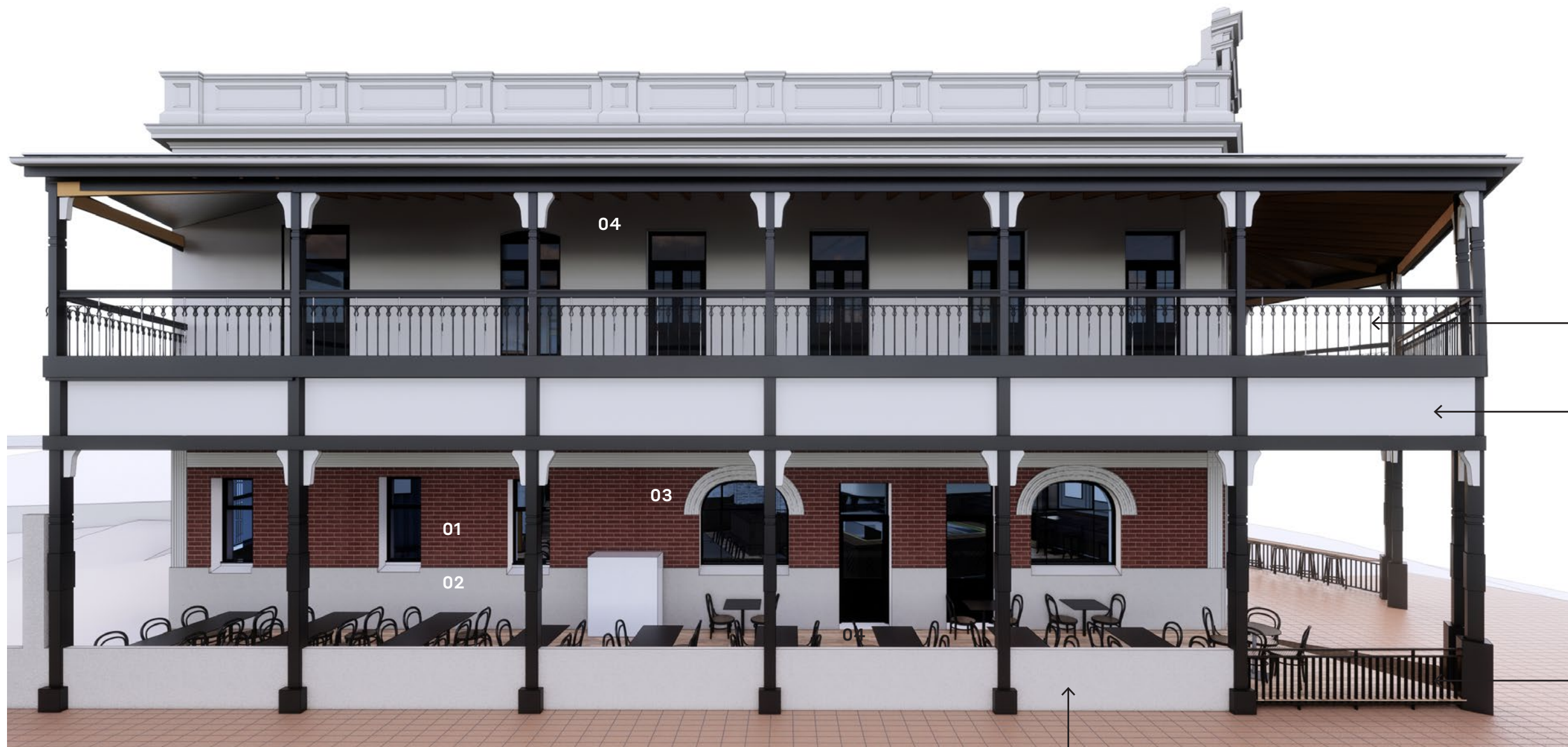
Existing balustrade to be retained, new clear panel applied at the back for compliance.
