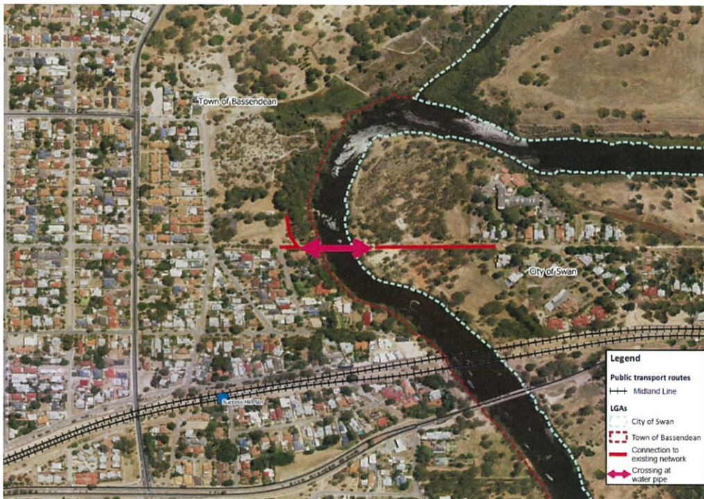
Figure 10 – Proposed water pipe pathway alignment
