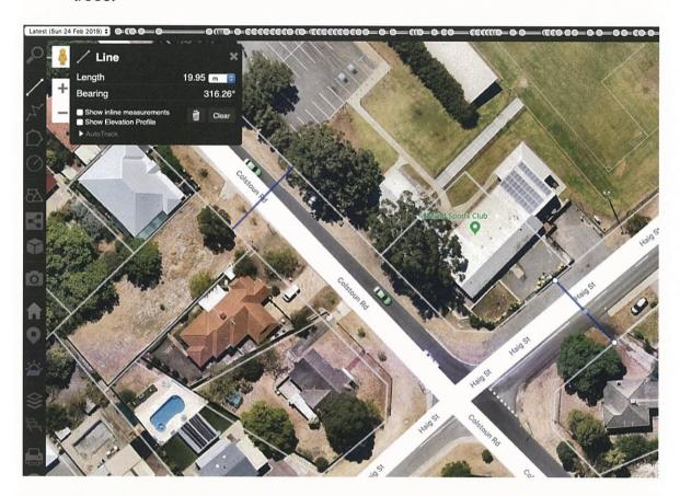
Figure 2. Ashfield aerial photo sample for road reserve widths.
