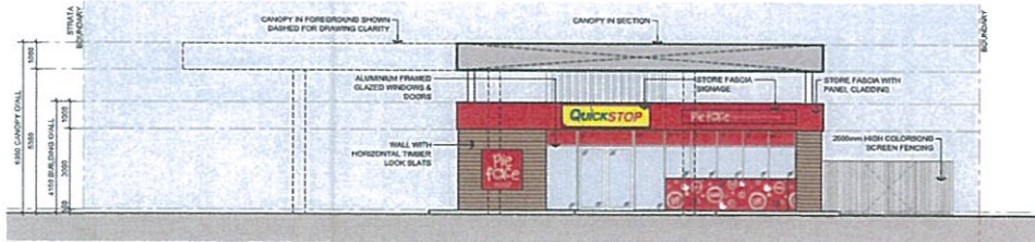
SOUTH EASTERN BUILDING ELEVATION (FRONT) SCALE 1:100
